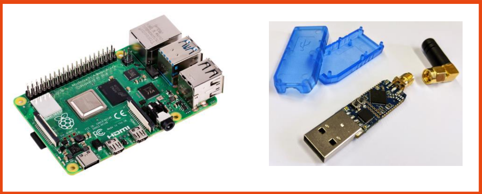
MCU - RASPBERRY PI AND GATEWAY
